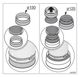
■ Attach the vent ducting to the exhaust socket, using e.g. a flexible hose and clips (available as an optional accessory).
